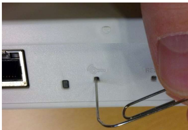
Figure 12 - Straightened paper clip used to enable the PGC button.
