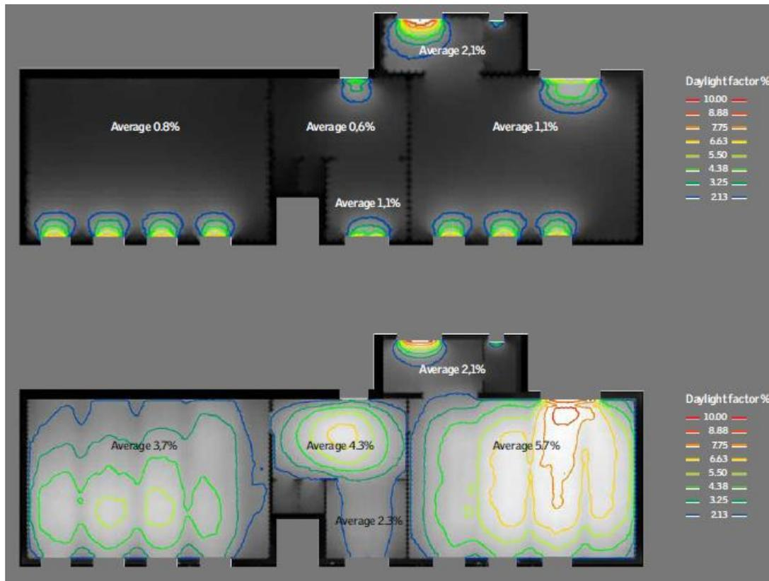
Fig. 3 The daylight factor analysis has been performed using the VELUX Daylight Visualizer, a software tool dedicated to daylighting design and analysis (more information at <http://viz.velux.com>). The upper part is existing classrooms, while the lower part shows the renovated classrooms and the effects of adding roof windows on the daylight levels and distribution.
