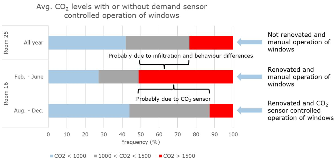
Fig. 5 Distribution of CO<sub>2</sub> concentration in the renovated and non-renovated classrooms. The blue colour shows CO<sub>2</sub> distribution below 1000 ppm; the red colour above 1500 ppm; and the grey shows concentration between 1000 – 1500 ppm.
