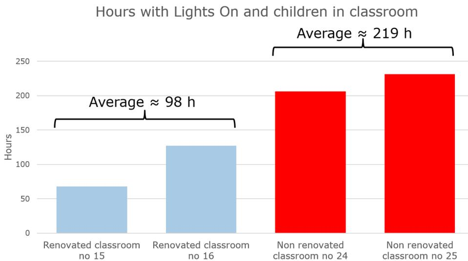
Fig. 4 Measured results of the electric lighting use and the switching patterns demonstrate that better daylighting performance have an impact on the behavioural switching patterns. In the bar graph, the renovated classroom is blue bars (classroom 15 and 16) and non-renovated classrooms is the red bars (classroom 24 and 25).
