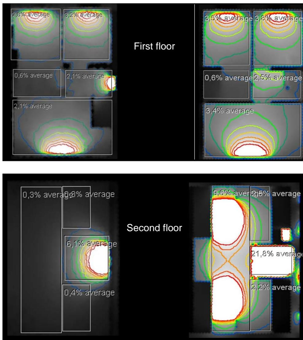
Figure 2. Daylight performance (daylight factor) for the room on first and second floor in the existing (left) and renovated (right) situation.
