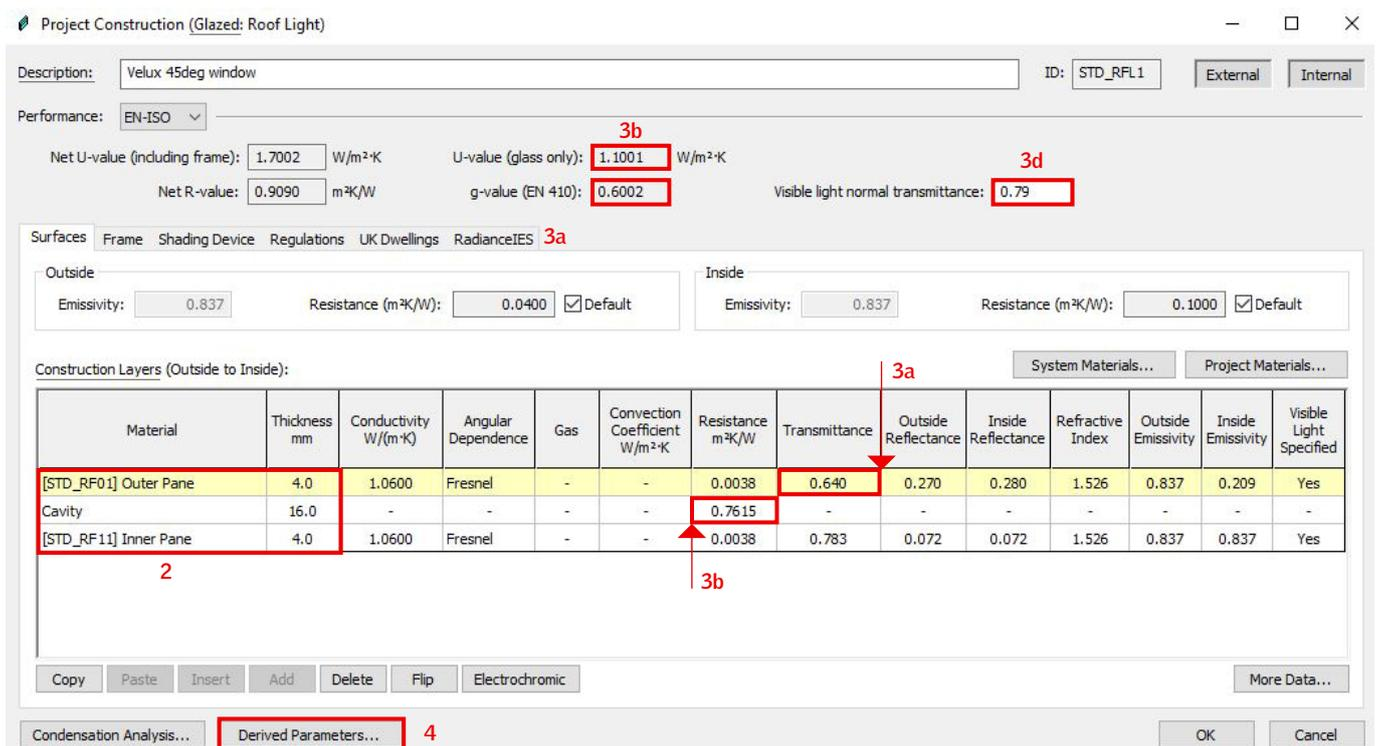
The screenshot shows the 'Project Construction (Glazed: Roof Light)' dialog box. The 'Description' field is 'Velux 45deg window'. Performance metrics include Net U-value (1.7002 W/m²·K), U-value (glass only) (1.1001 W/m²·K), Net R-value (0.9090 m²K/W), g-value (EN 410) (0.6002), and Visible light normal transmittance (0.79). The 'Surfaces' tab is active, showing 'Outside' and 'Inside' properties. The 'Construction Layers (Outside to Inside)' table is highlighted with red boxes and arrows:
