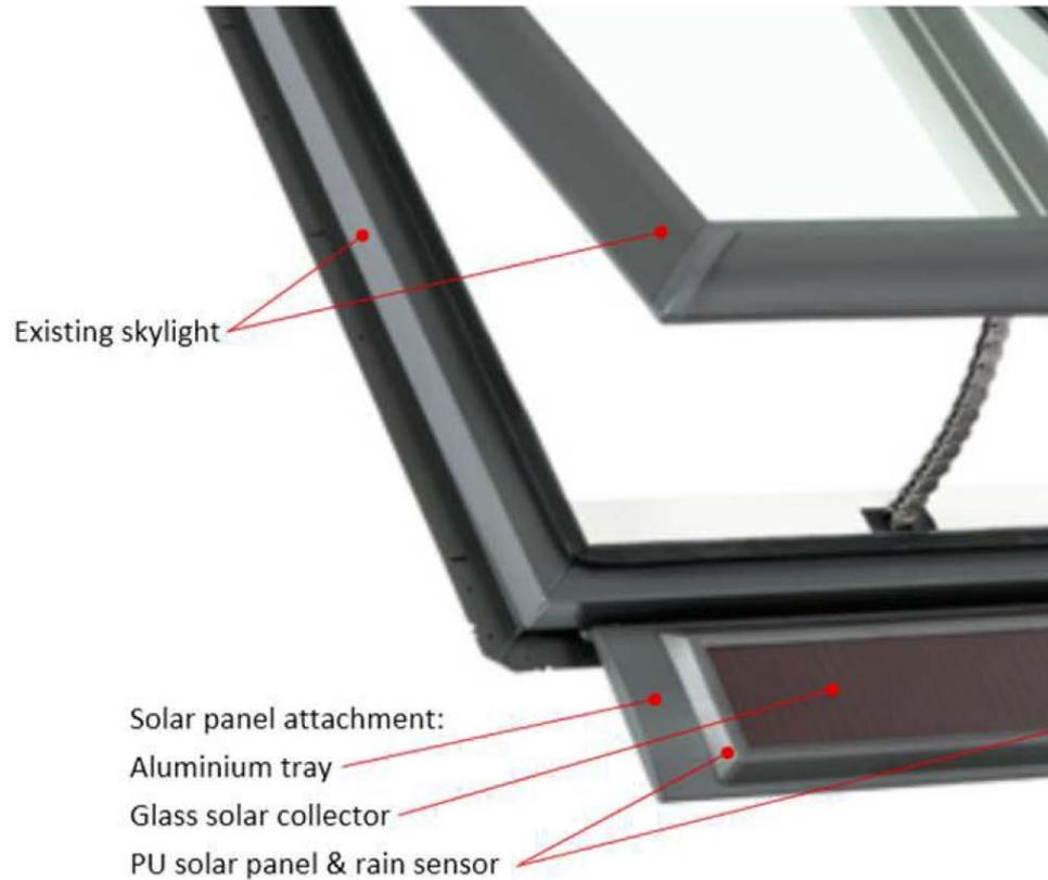
**Figure 1. Skylight with solar panel attachment**
