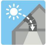
The  $\boldsymbol{rigid}$  tunnel is ideal for distances between roof and ceiling from 0.9 to 1.7 m - with extension sections up to 6 m.
