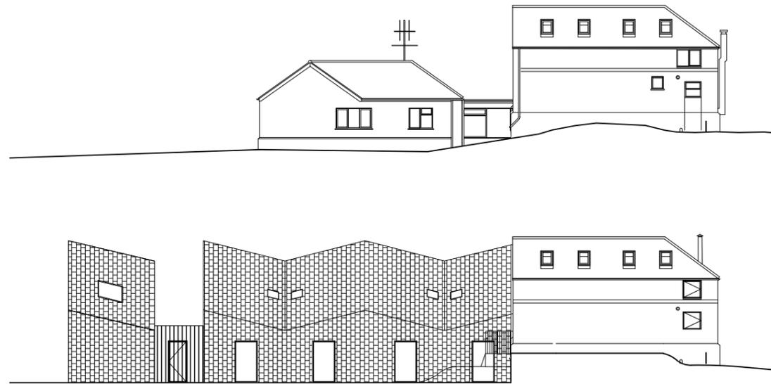
Facade before and after refurbishment. The old building has been torn down and replaced by a new wing with bedrooms. The old barn has been refurbished in a very gentle manner, with minimal alterations of the facade. Broken roof tiles were replaced with ones with patina.
