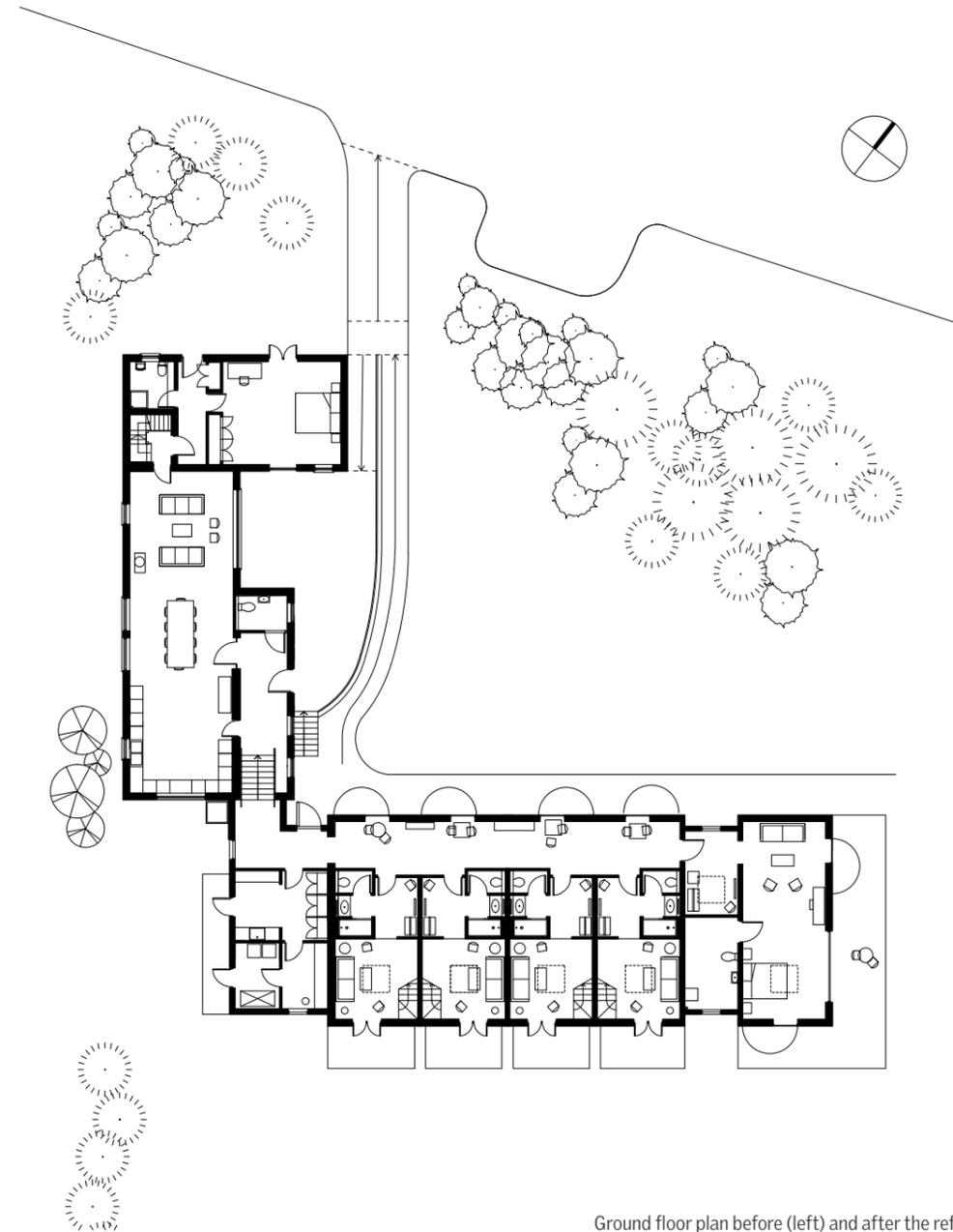
Ground floor plan before (left) and after the refurbishment. Old barn and bedroom wing are connected with a one-storey high volume with stairs leading up to the living area. The corridor with shelves and cosy reading corners at the facade opens with a full-height window towards the garden. The last unit, larger than the others, is separated by a low, black-painted element to break the length of the building.
