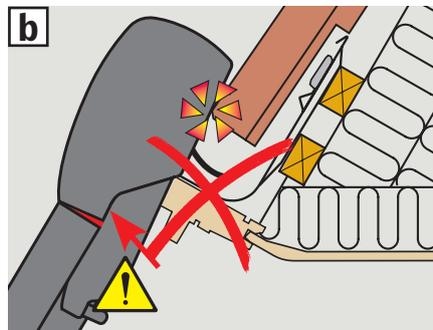
**ENGLISH:** Lower the roller shutter top casing as much as possible. Do **not** press the top casing against the roofing material [a](#), [b](#). Pull cable through hole on window top cover. Fit securing screws after installing the roller shutter top casing [c](#), [d](#).
