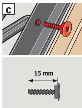
**ENGLISH:** Push side channels into position [a](#) and lay down on side covers [b](#). Attach opening restrictors to side covers with screws [c](#).
