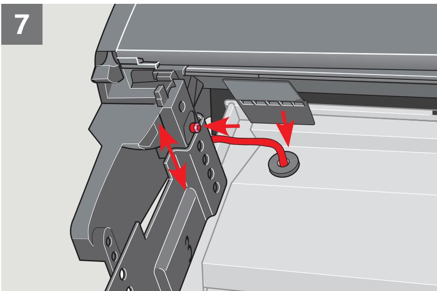
**ENGLISH:** Lower the roller shutter top casing as much as possible. Do **not** press the top casing against the roofing material **[a]**, **[b]**. Pull cable through hole on window top cover.
