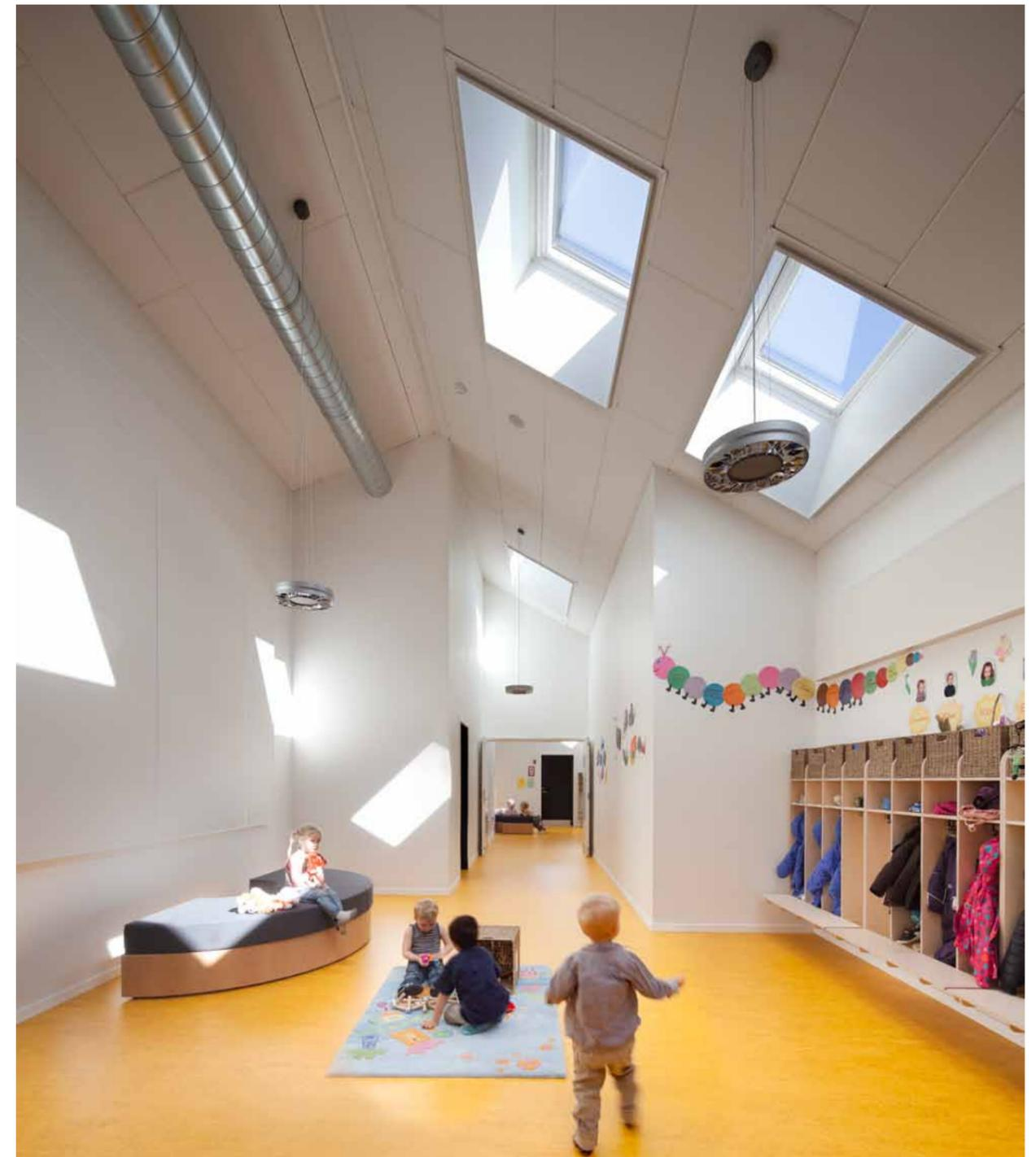
Intelligently controlled sun screening and window opening make the house flexible, allowing the flow of daylight and fresh air to adapt continuously to the weather conditions outside and the needs indoors. Solhuset is built of sound materials that have minimal impact on the indoor climate. Vertical windows in the south-east and south-west facades and roof windows let in more than three times as much light as in a traditional house.
