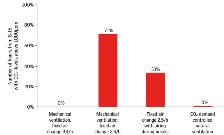
The comparison of the results shows that demand-controlled natural ventilation with CO<sub>2</sub> sensors provides much better air quality to the room than the fixed air change of 2.5 (calculated according to BR 2010). Demand-controlled natural ventilation is operated by CO<sub>2</sub> sensors installed in each classroom. The opening of the windows is controlled by two setpoints:
