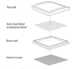
Mounting of blinds is done most conveniently during the rooflight installation process.
