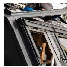
7 Transverse gutter • lacquered aluminium • colour: grey • ensures drainage between top and bottom row of windows
