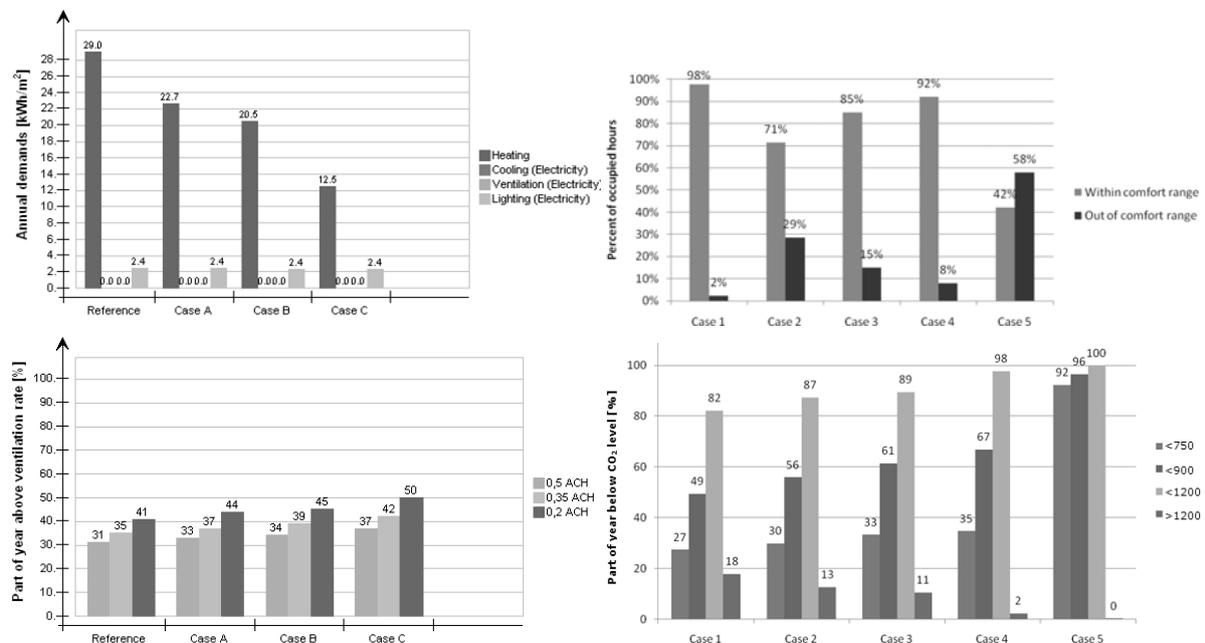
Figure 2. Results as presented in the comparison report. Energy demands (upper left), thermal comfort (upper right), ventilation rates (lower left) and CO<sub>2</sub> levels (lower right)
