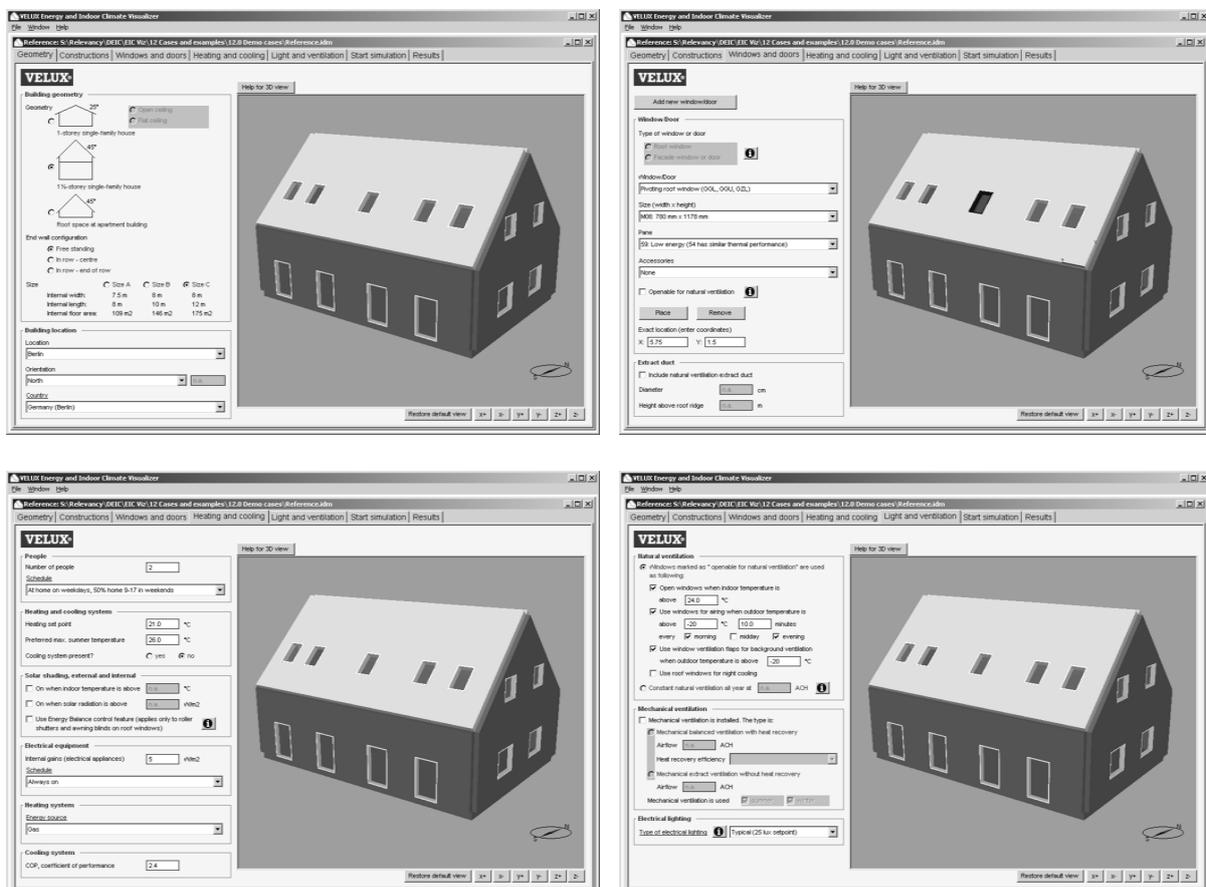
Figure 1. The user interface of the Energy and Indoor Climate Visualizer with the Geometry tab active (upper left), Windows and doors (upper right), Heating and cooling (lower left) and Light and ventilation tab (lower right)
