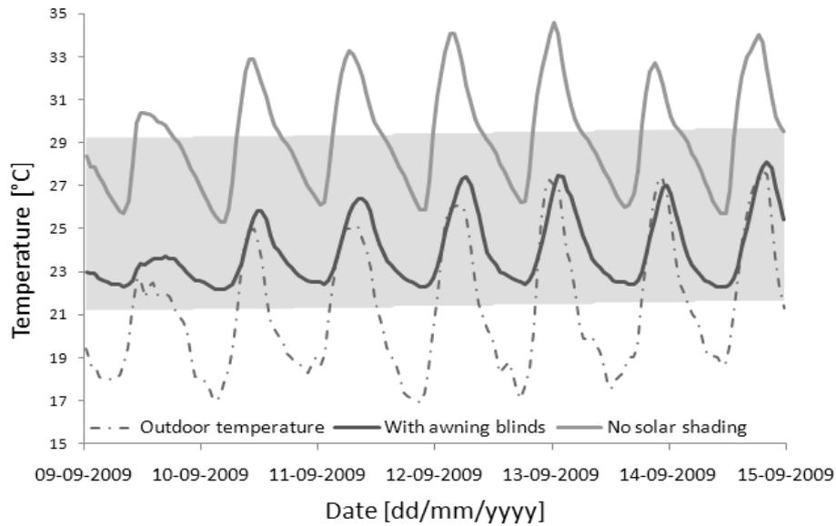
Figure 3. Presentation of operative temperature of the simulations with the comfort range (solid grey) based on running mean outdoor temperature.
