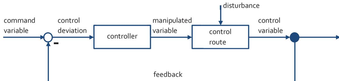
Figure 1: flow chart of an automated technical control
