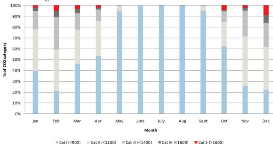
Figure 1: Measured CO<sub>2</sub> concentration in the kitchen/living room of LichtAktiv Haus, Germany. The data is categorized according to the Active House Specification
