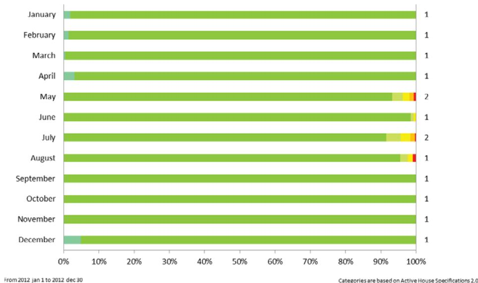
Figure 2: Measured indoor temperature in the kitchen/living room of LichtAktiv Haus, Germany. The data is categorized according to the Active House Specification. The number on the right side of the figure is the Active house category achieved for each month (max 5% of the time can exceed the category)
