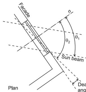
Figure 1 Dead angle and angle of the sun beam incidence  $\theta_1$
