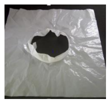
5 Vapour barrier collar Vapour barrier collar BBX is supplied with the sun tunnel to ensure a tight connection between the sun tunnel and the existing vapour barrier of the house.
